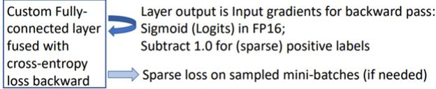
Figure 3. Optimized classifier with fused linear and cross entropy loss backward layer and optional sparse loss computation.
