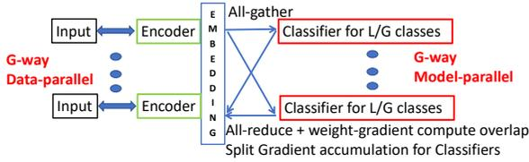
Figure 5. Hybrid data-model parallel architecture with all-reduce communication overlapped with weight gradient computation and split gradient accumulation for classifiers.
