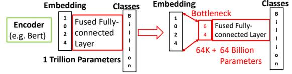
Figure 4. Use of a bottleneck layer to optimize classifier parameter memory and compute requirements.
